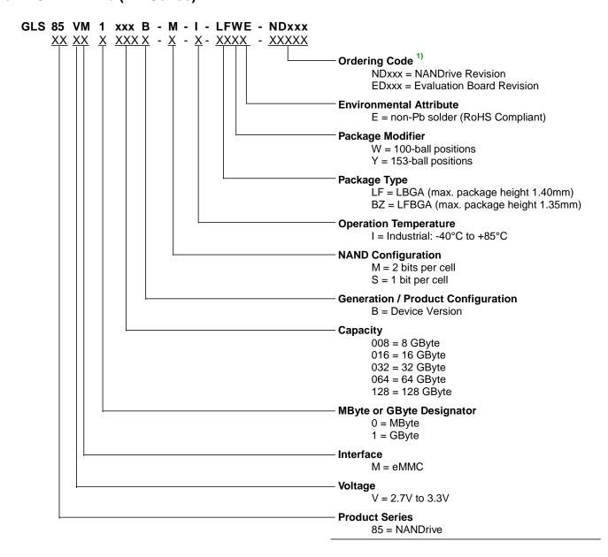
1) Note that the top side marking on the package typically does not include ordering codes (e.g. NDxxx), unless it is a special C-SPEC (custom specification) which is required by the end-customer to be marked on the device.
